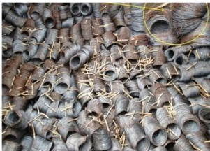
× Loose condition due to non – rigid straps/packaging
